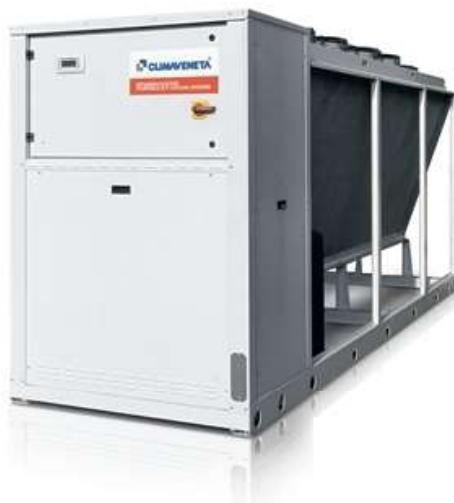
**Outdoor unit with heat pump for the production of chilled/hot water with hermetic rotary scroll compressors dedicated to the use of R410A, axial fans, plate heat exchanger, condensing coil with copper tubes and aluminum fins and thermostatic or electronic expansion valve, according to the version. The range is composed by units equipped with two compressors in a single-circuit configuration.**
