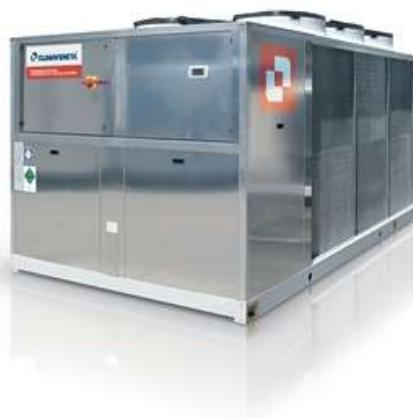
**Outdoor reversible unit for the production of chilled/hot water with hermetic rotary Scroll compressors, ozone-friendly refrigerant R410A, axial-flow fans, copper tubes aluminum fins air coils, braze-welded plate-type exchanger and thermostatic expansion valve. External panels in pre-clad sheet steel and base in galvanised steel with paint finish. The range is composed by units equipped with four compressors in tandem configuration on two independent refrigerant circuits.**
